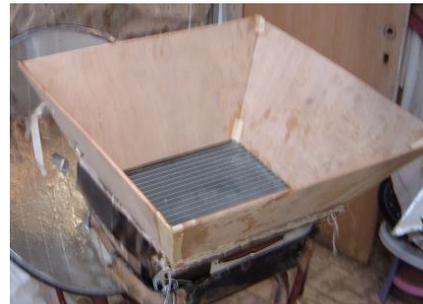
the glue is nearly dry, stand the panels gently bends of the side flaps, and temporarily tape the last two segments tightly together with elastic material. This will allow these corners to separate slightly when the collectors are folded flat, but pulls the corners together when unfolded.
